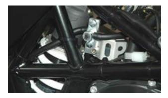
6. Route the fuel line similar to the photos below. Routing will be from fuel taps (LH & RH sides) through the bottom mounting brackets to the 'T' section and then to the tap block onto the fuel adapter assembly. Ensure the fuel lines do not kink.
