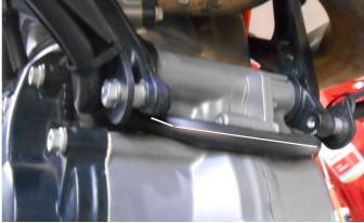
7. Install the tank mounting brackets (LH & RH bracket, top bracket and both standoff bolts) with the associated bolts, washers and spacers (bottom brackets).
