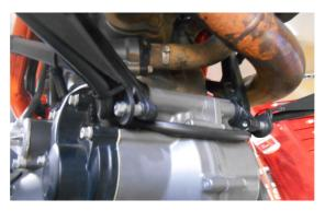
Note;- Use the supplied spacers for the bottom LH and RH brackets
